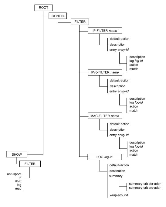
Figure 25: Filter Command Structure
